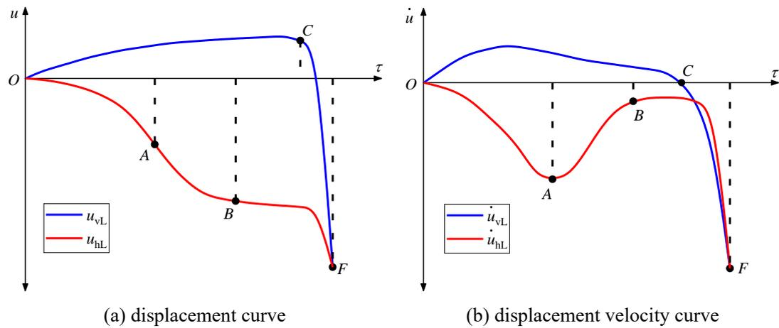
Fig. 11 Variation trends of early-warning indexes for side-column buckling collapse mode B.
