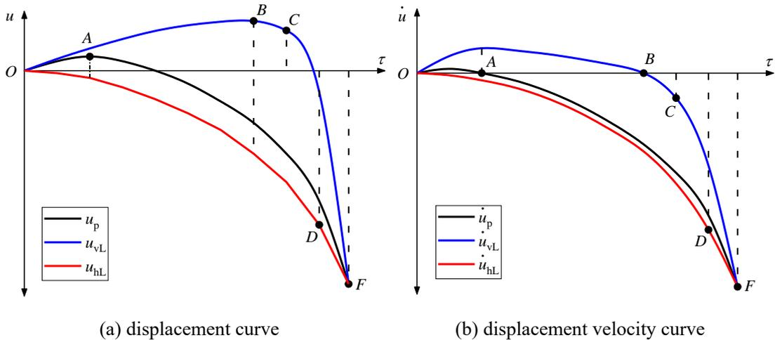
Fig. 10 Variation trends of early-warning indexes for side-column lateral collapse mode A.
