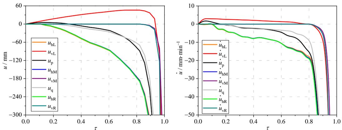
(a) Side-column lateral collapse mode A
