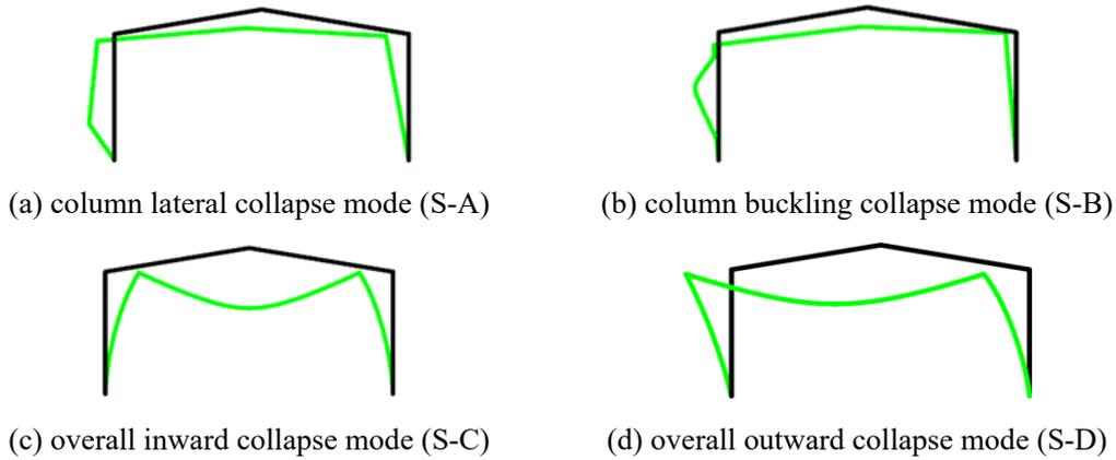
322 Fig. 7 Collapse modes of single-span steel portal frames [26].
